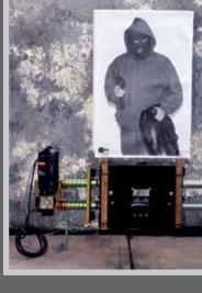
**INSTALLATION:** Because the drive components (track, motor & trolley) are not balistically protected, the entire system is usually installed behind a knee wall. All of the drive components simply clamp on to the track, so the system can be taken down quickly and put away to prevent vandalism or theft on unsecured ranges. Even so, all drive components are protected from the weather so they can be left out in harsh conditions with no problem.
