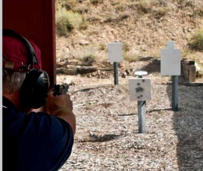
Action Target automated steel can be used for long distance sniper work and have your target or multiple targets reset each time they fall after a hit. They can also be programmed to come up at varying times in a training scenario. Short range targets have various training possibilities as well. They can be used for automated qualification drills and even provide scoring printouts of the course detailing times of engagement in addition to the basic score.
