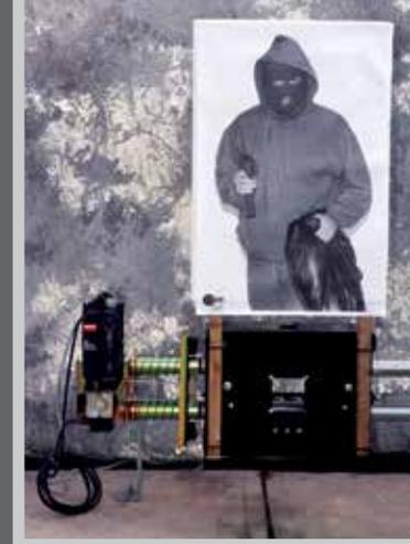
**INSTALLATION:** Because the drive components (track, motor & trolley) are not ballistically protected, the entire system is usually installed behind a knee wall. All of the drive components simply clamp on to the track, so the system can be taken down quickly and put away to prevent vandalism or theft on unsecured ranges. Even so, all drive components are protected from the weather so they can be left out in harsh conditions with no problem.
